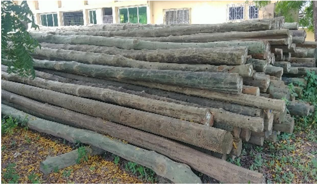
PIC 5; Low tension Poles
